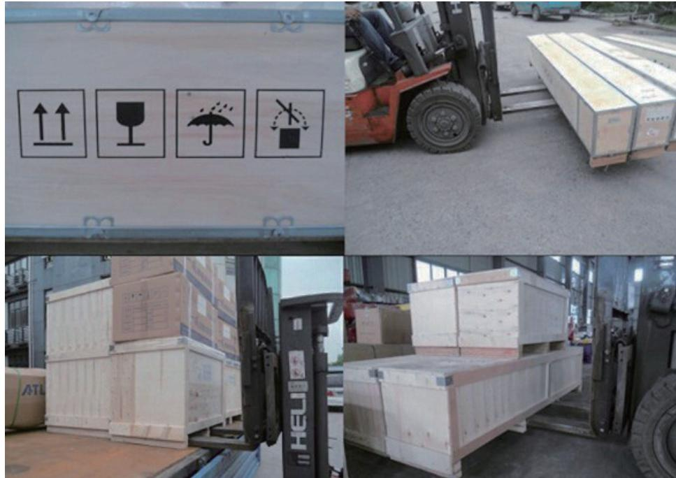
(Note: The maximum load capacity of the forklift shall be greater than 0.5 t.) [The figure shown above is for reference only.]
