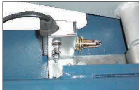
Fig. 9 (Limit switch of sub lift)
