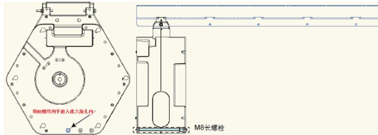
[4] Insert the subsequent reel into the lifting beam in sequence, and align the locating pin protruding from the left side of the housing with the locating hole on the right side of the left reel. Then pat to insert it tightly and tighten the M8 long bolt.
