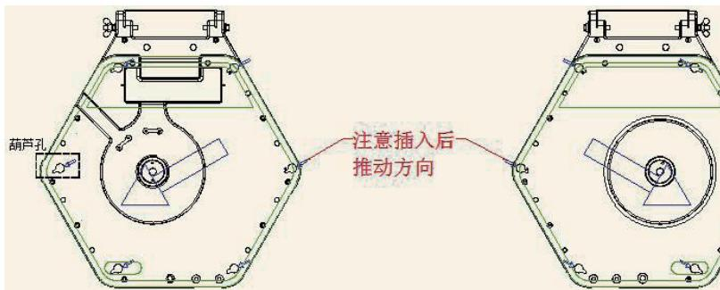
5.2 In this way, install the end caps respectively at both ends of the combined reel. Now the fixing and fitting of the reel is completed.
