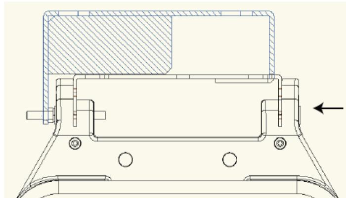
[3] Open the end cap accessory bag, take out the M8 nut, insert it into the left hexagonal hole of the reel, and tighten the M8 long bolt.
