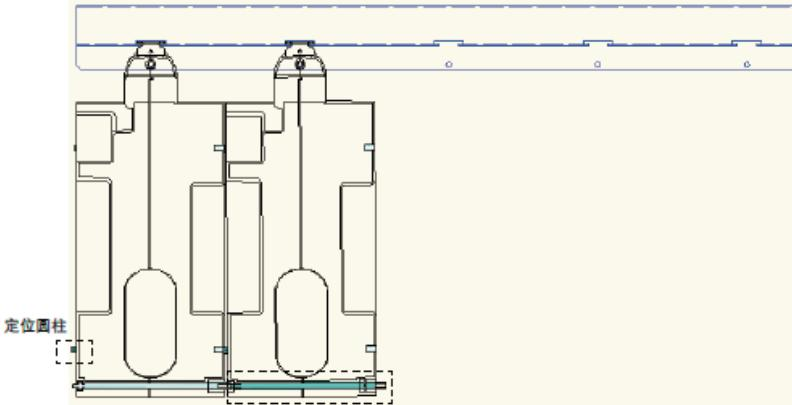
[5] After all the reels are installed in sequence, arrange the M6 spring washer removed previously onto the stand bolt as shown in the figure, and then tighten it with the M6 butterfly nut (so that all the reels can be fixed).
