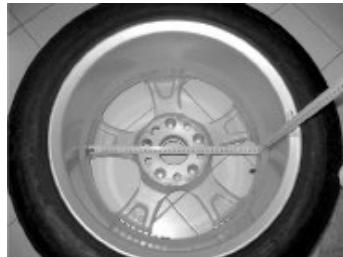
Fig. F3.3.1 Example of manual measurement of outer diameter (da2) in ALS1/ALS2 mode
