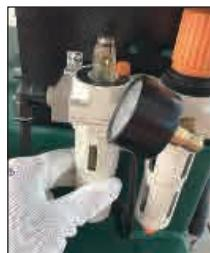
Check the lubricating oil level every day, and open the oil cap to add oil when necessary. Attention: It is forbidden to use lubricating oil exposed to air for a long time.
