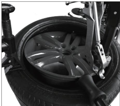
3.11 As shown in the figure, press the tire pressing roller and the tire pressing block below the rim edge, so that the tire is not exposed as recommended, and mount the upper tire.
