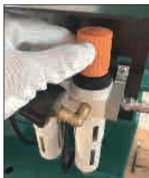
Pull out the cover, rotate the adjustable pressure. The pressure setting range is 8-10 bar.
