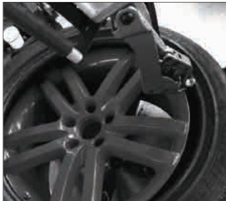
3.10 Rotate the rim driven by chuck clockwise, and mount the lower tire first.
