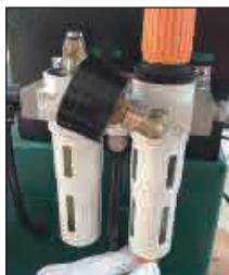
Regularly check the water level of the steam-water separator. Do not exceed 50% height of the separator. If necessary, turn the locking button to drain water manually.
