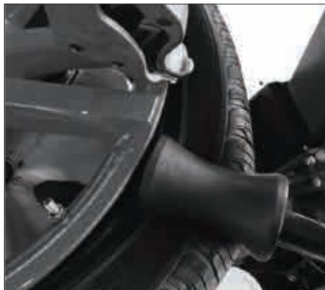
3.2 Pull down the lifting manual valve of the hexagonal rod so that the mounting head is 2 mm away from the top of the rim.
