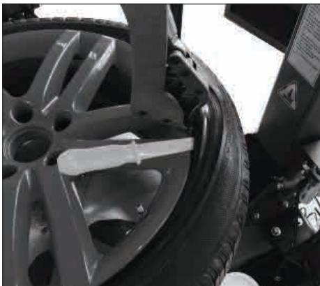
3.6 Insert the plastic crowbar and step on the revolving pedal so that the chuck drives the tire to rotate clockwise, thus separating the single-side tire.
