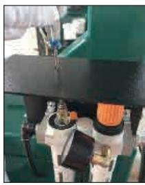
Check the lubrication conditions every day to ensure that the lubricating oil drips into the oil atomizer when stepping on the pedal. If necessary, use a screwdriver to adjust the adjusting screw of the oil atomizer.
