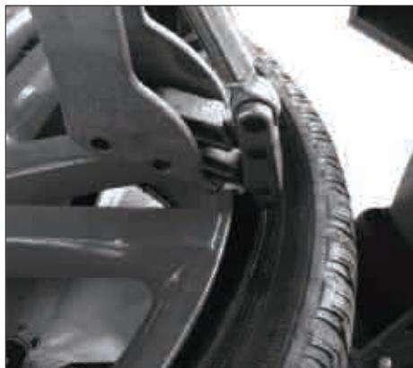
3.4 Press the manual valve until the tire dismounting hook penetrates into the inner part of the tire.
