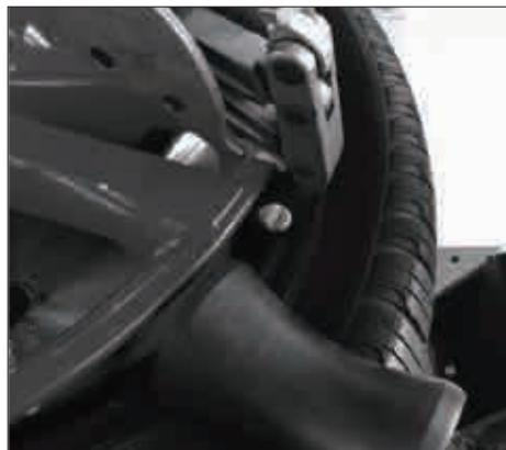
3.3 Pull down the manual valve of the mounting head, and extend the tire dismounting hook into the tire.
