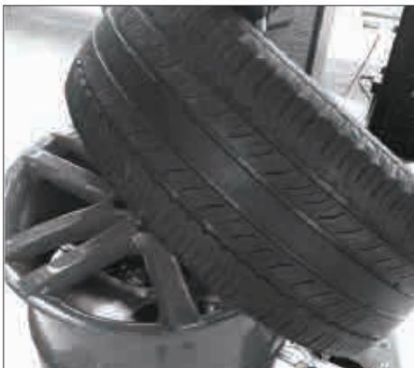
3.8 Step on the revolving pedal so that the chuck drives the tire to rotate clockwise; at this moment, the lower tire opening of the tire is separated from the rim.
