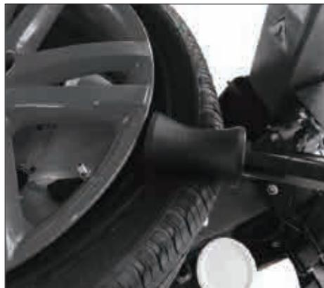
3.1 Press the tire with the tire pressing roller of the auxiliary arm as shown in the figure.
