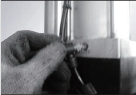
Fig. 7-7 Install the elbow attached to the pipe to the cylinder as shown in Fig. 7-7.
