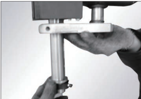
Fig. 7-9 Remove the fixing shaft of auxiliary arm tumbler as shown in Fig. 7-9.
