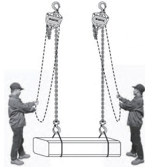
9. It is prohibited to lift weights with two or more lever blocks together.
