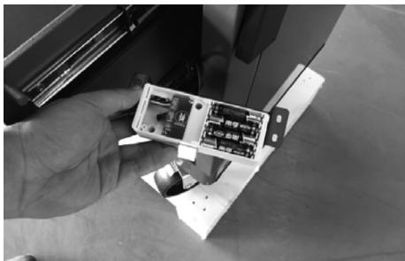
Step 5: Install the lock unit, adjust its position, and install the screws to rightmost ends of the holes.
