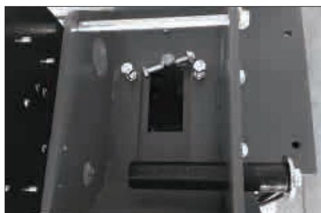
a. Dismount the column shaft on the rear inclined arm seat to be mounted.
