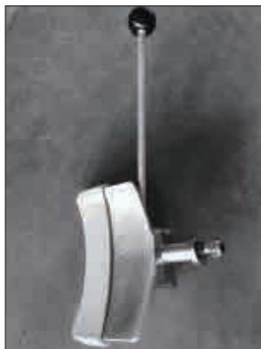
1 Take out the tire pressing shovel and dismount the spacer and locking nut on the shaft of the tire pressing shovel.
