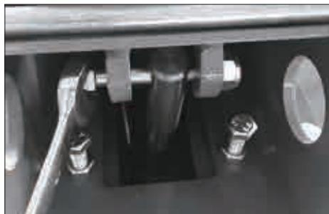
f. Connect the cylinder rod to the column with a bolt.
