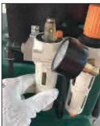
Check the lubricating oil level every day, and open the oil cap to add oil when necessary. Attention: It is forbidden to use lubricating oil exposed to air for a long time.
