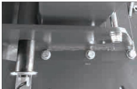
e. Insert the column shaft into the column, and fix it with the stud and washer.
