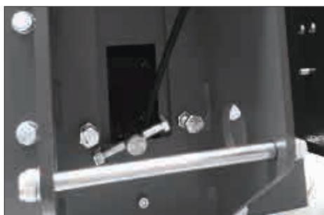
b. Put the air pipe on the column through the square groove on the rear inclined arm seat.
