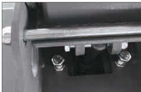
g. Adjust the set screws on both sides of the column.
