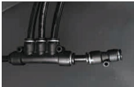
d. Connect the air pipe on the column to the 8-to-6 joint, and remount the siding plate.
