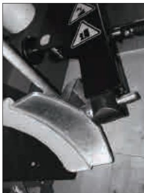
2 Penetrate the tire pressing shovel shaft into the shovel arm crank shaft.
